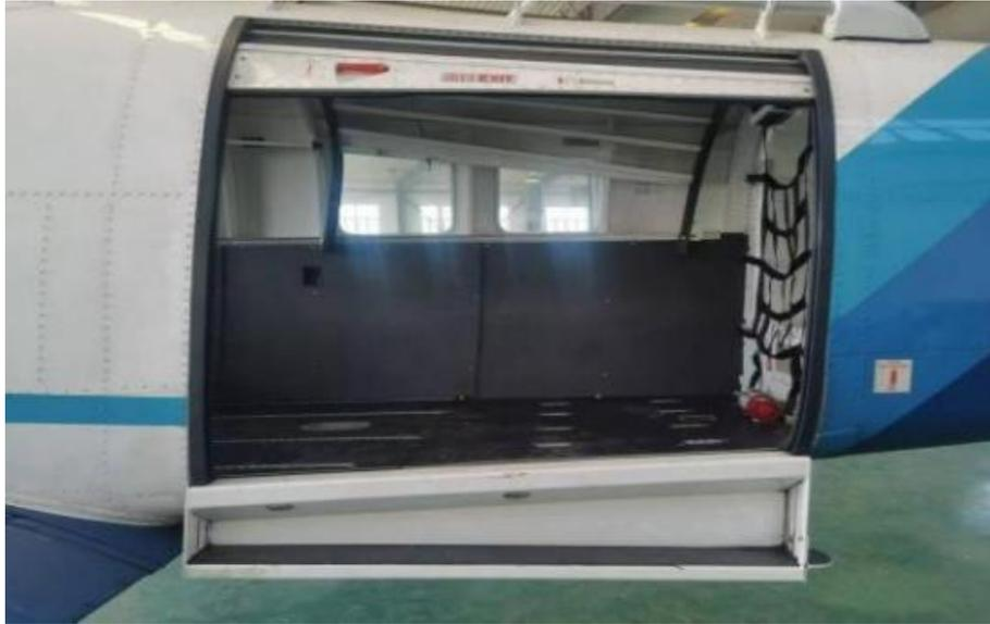
The geometry of the exit door of the P750 is 48in-50in wide and 41.3in tall upstream along the fuselage and 39.3in tall at the downstream location. Aircraft are all CCAR-91 and CCAR-136 certified and equipped with seat belts and will be operated in full compliance with China's applicable air regulations.
